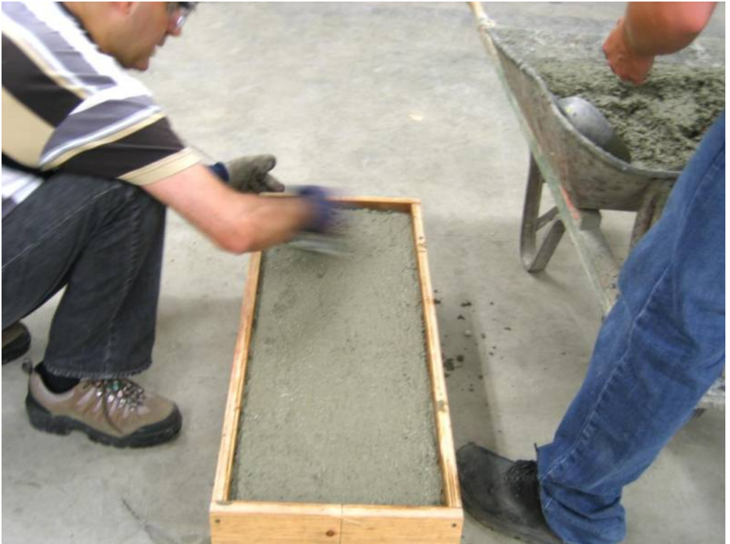
Figure 9: Filling the box with fresh concrete.
