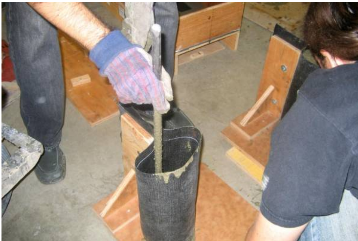
Figure 21: Compacting fresh concrete using the standard rod.
