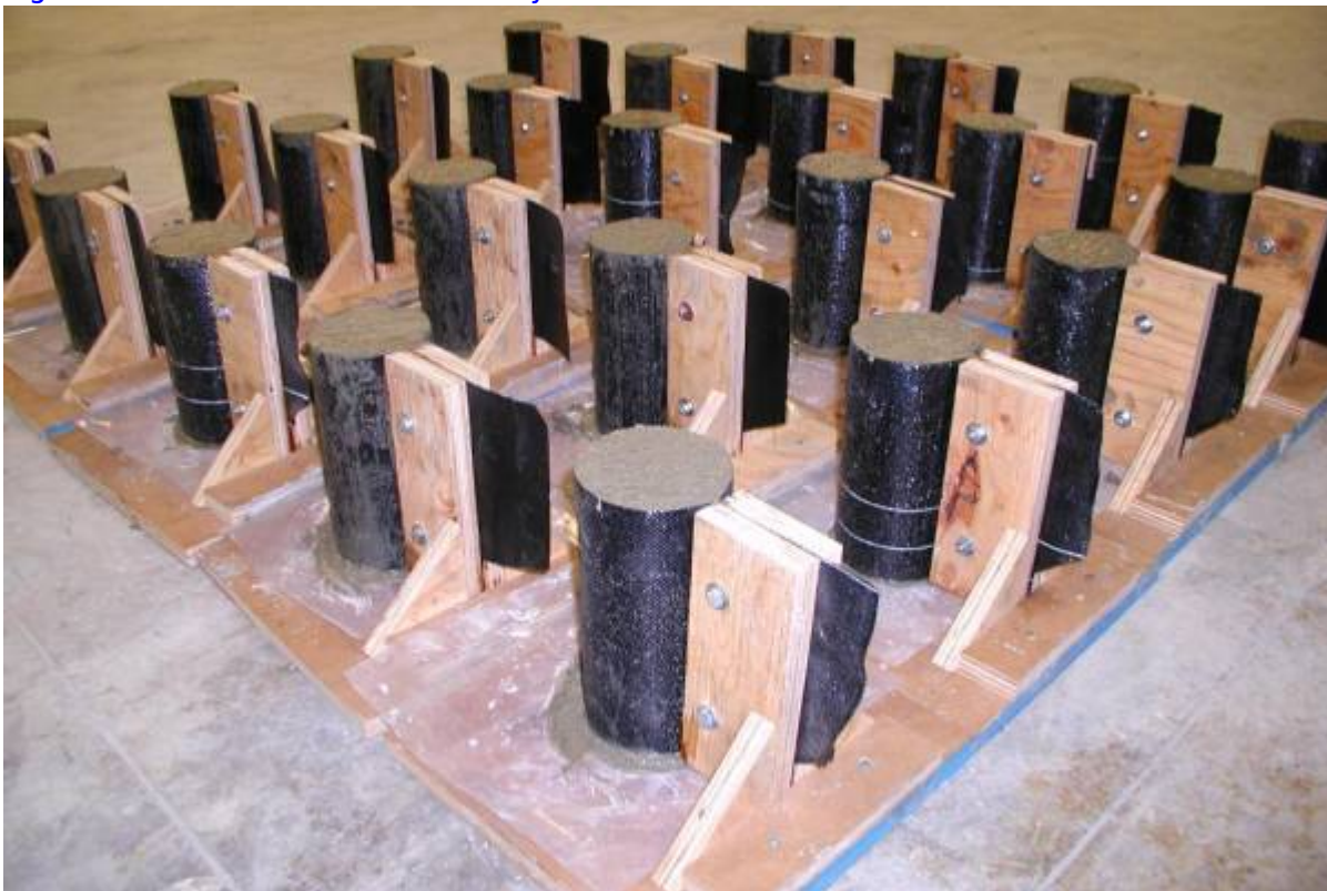
Figure 35: Fabric-formed cylinders after casting.
