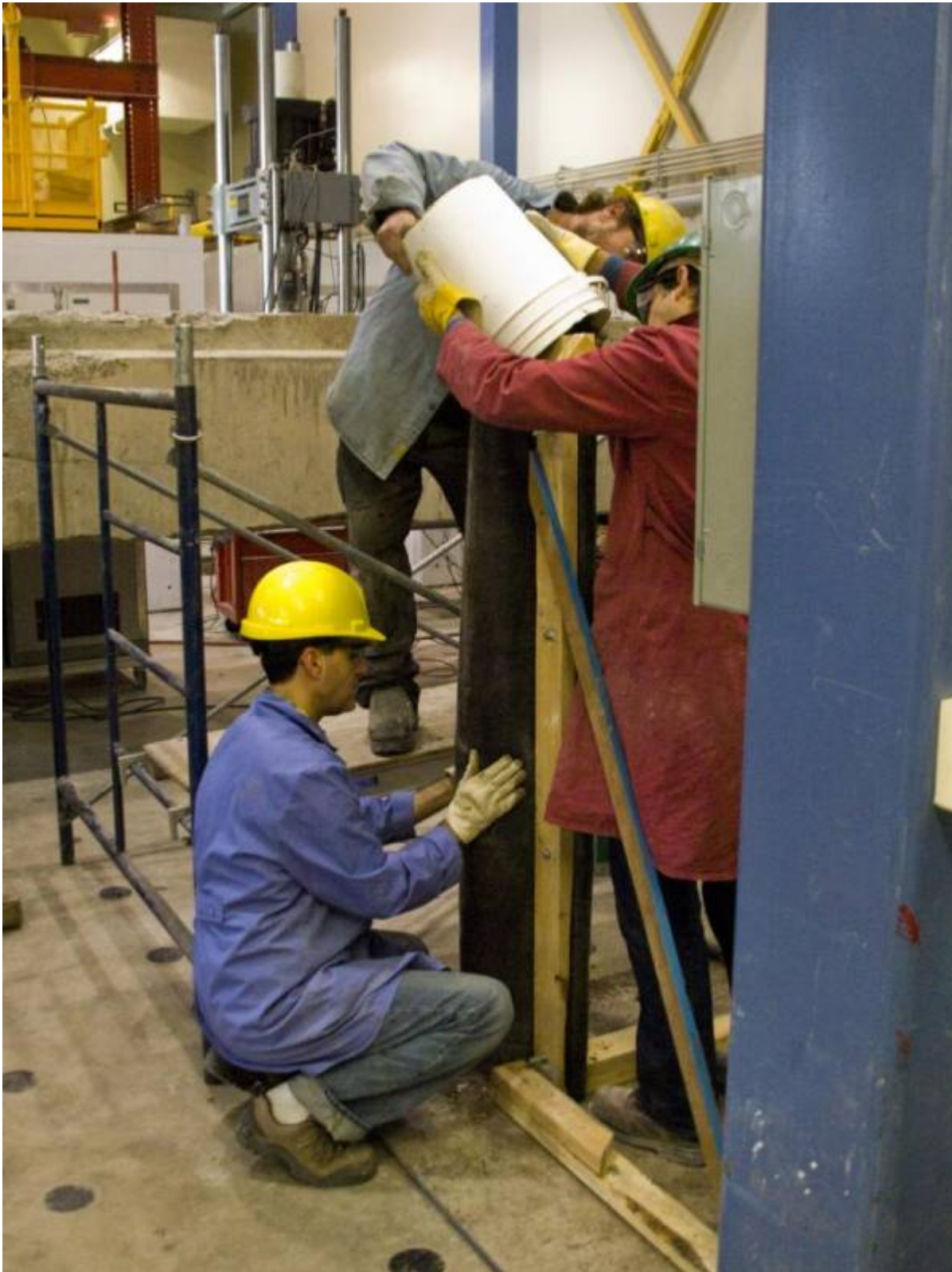
Figure 47: casting of column in fabric formwork.
