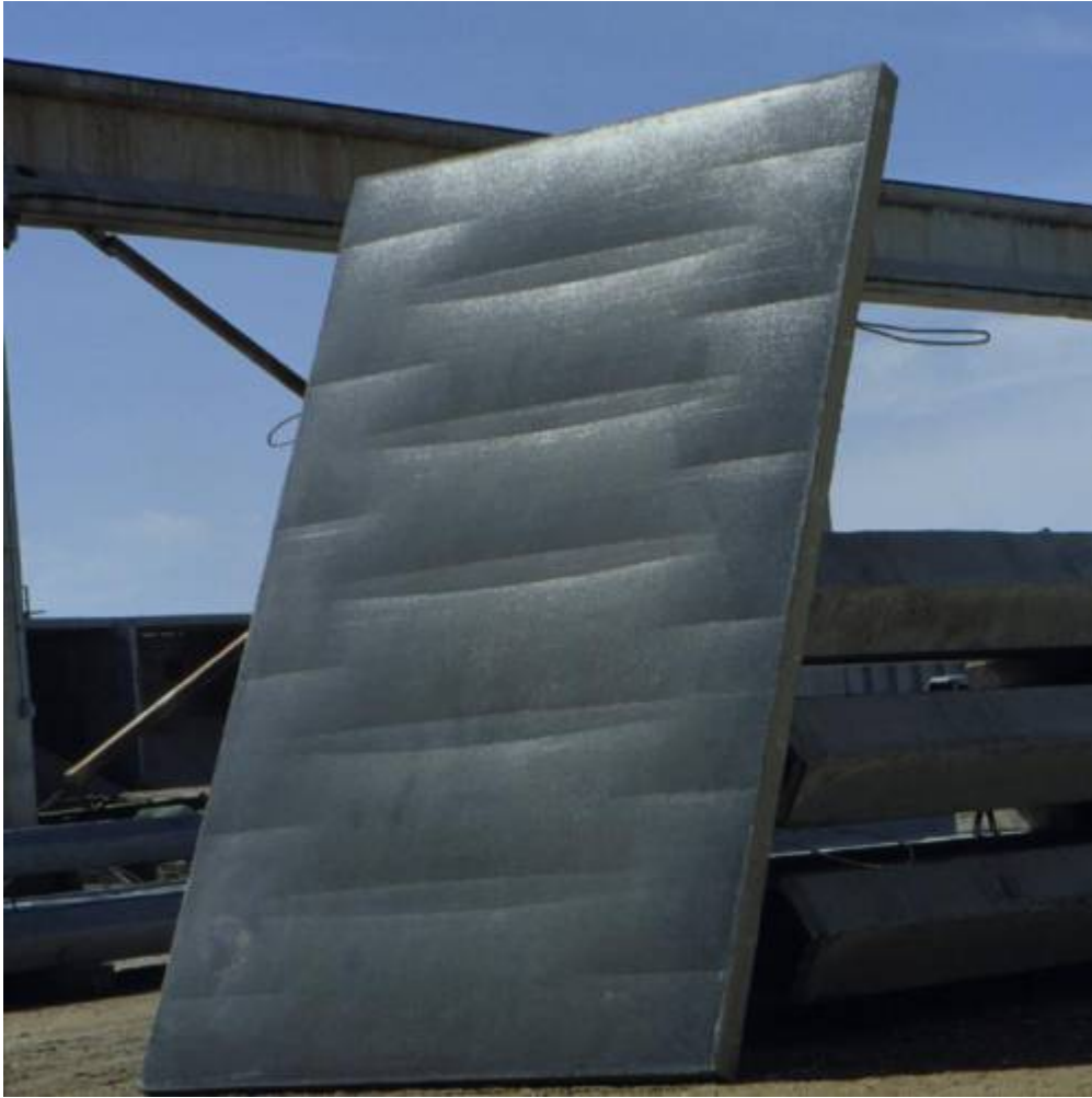
Fig. 10. Completed full scale concrete wall panel.
