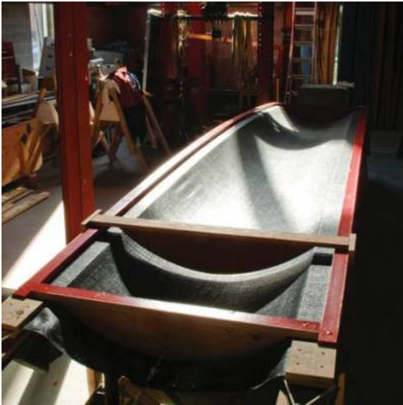
Fig. 33. Fabric mold stretched lengthwise in frame to form double curvature...
