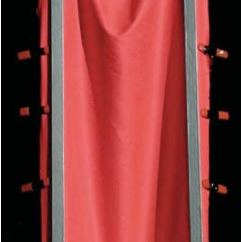
Fig. 42. Hanging sheet of fabric used as mold to produce thin-shell wall panels.
