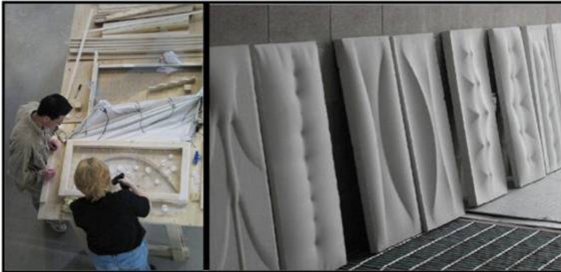
Fig. 1. Model formwork and completed plaster cast.
