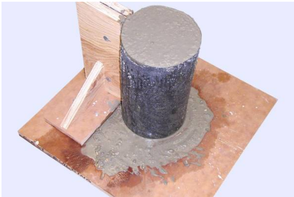
Figure 22: Fabric mold filled with fresh concrete.
