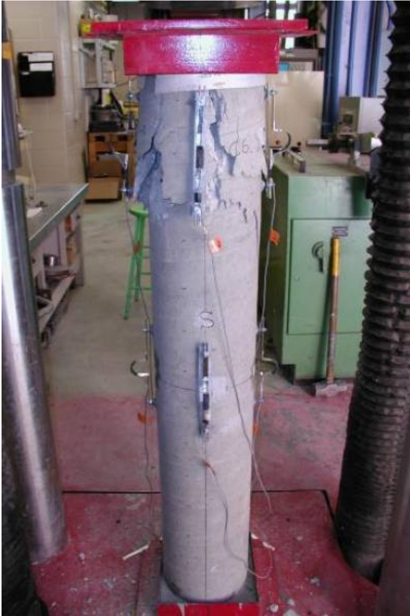
Figure 65: Column CT-NC-2 after failure.
