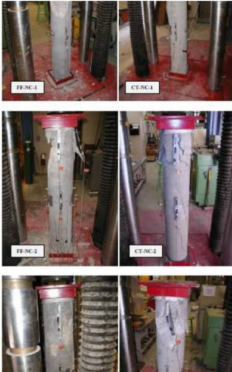
Figure 65: All columns after failure.
