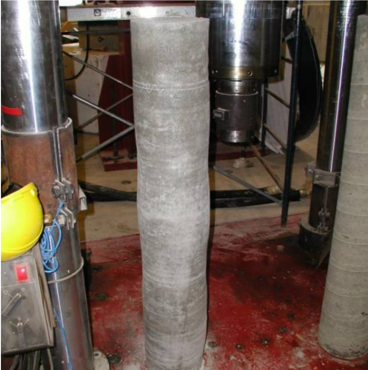
Figure 67: Bulged concrete column.
