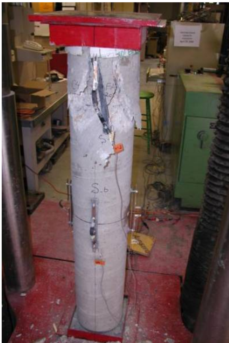
Figure 65: Column CT-FAC after failure.
