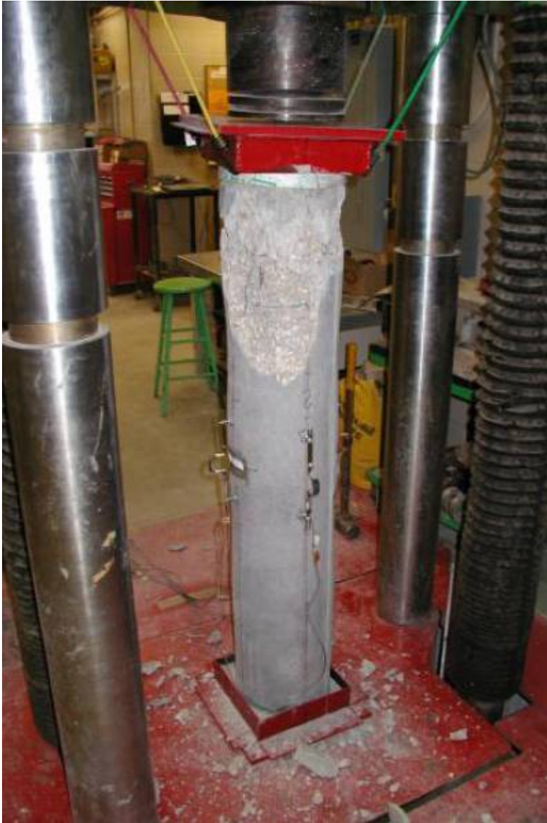
Figure 65: Column FF-NC-1 after failure.
