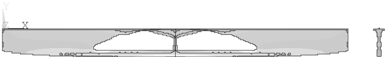
Figure 8.14 Front and side views of the optimized beam at generation 72. As before, there is only one mirrored pinch point.
