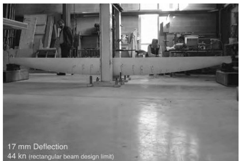
Figure 3.9 Photographs of destructive testing at C.A.S.T, Canada. A fabric formed beam is subjected to a three point bending test.
