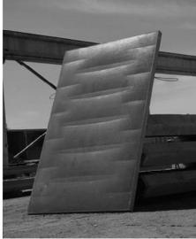
Figure 2: Full-scale formwork and completed concrete panel (C.A.S.T. photos).
