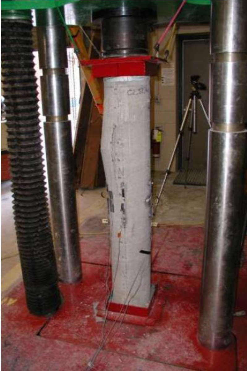
Figure 65: Column CT-NC-1 after failure.
