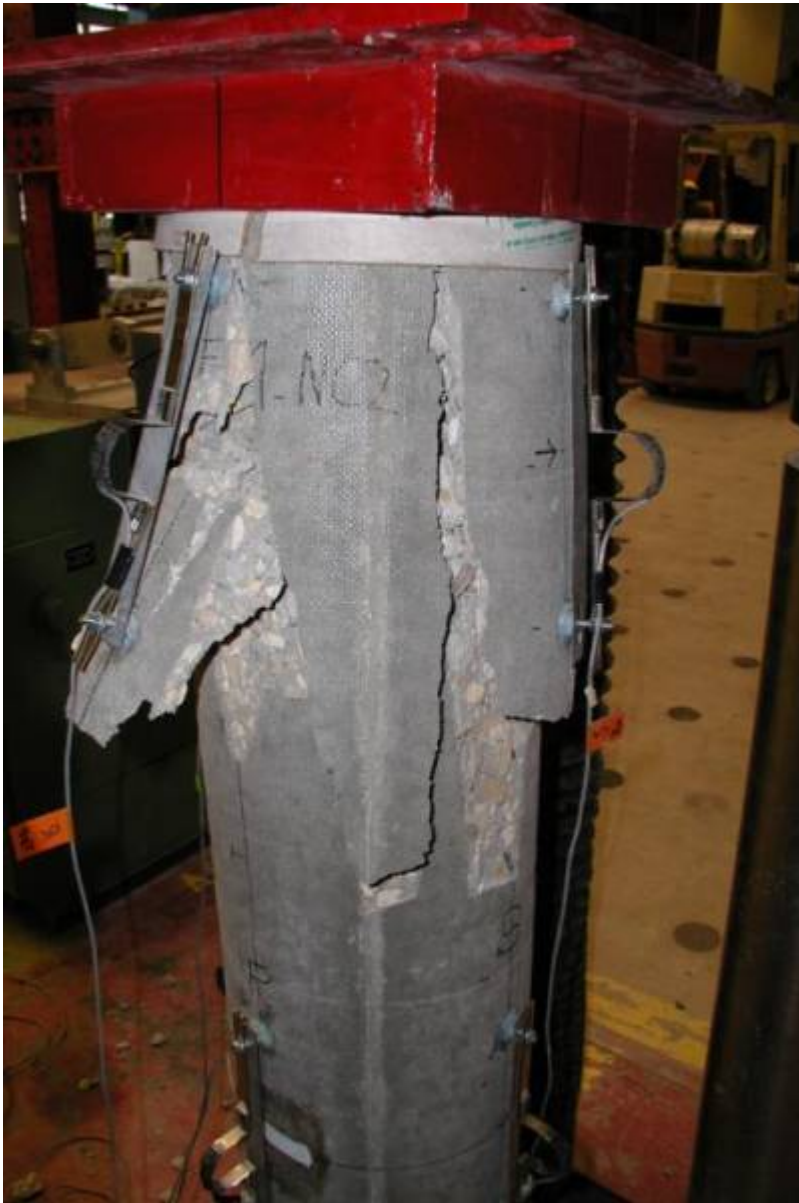
Figure 64: Column FF-NC-2 after failure.
