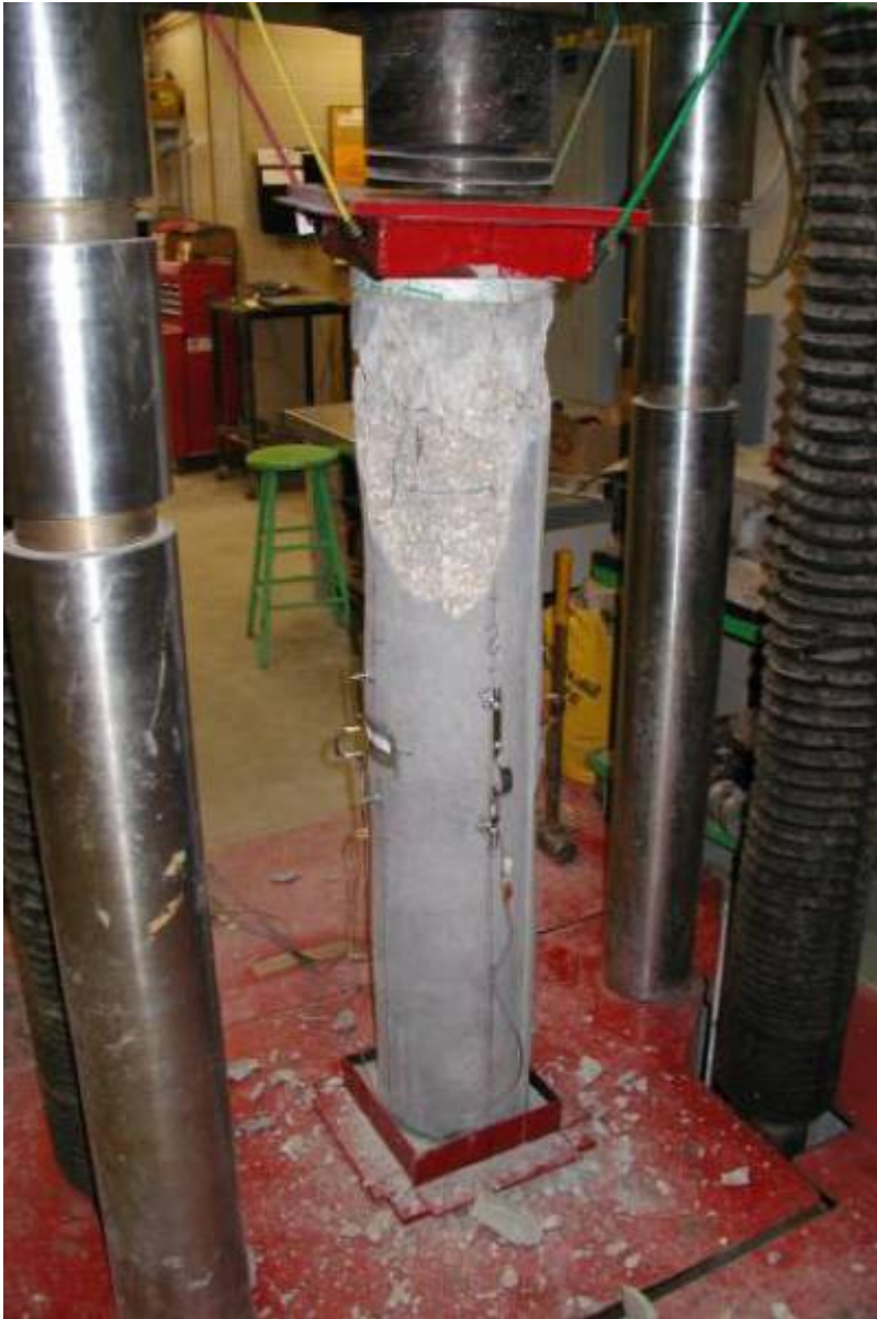
Figure 65: Column FF-NC-1 after failure.
