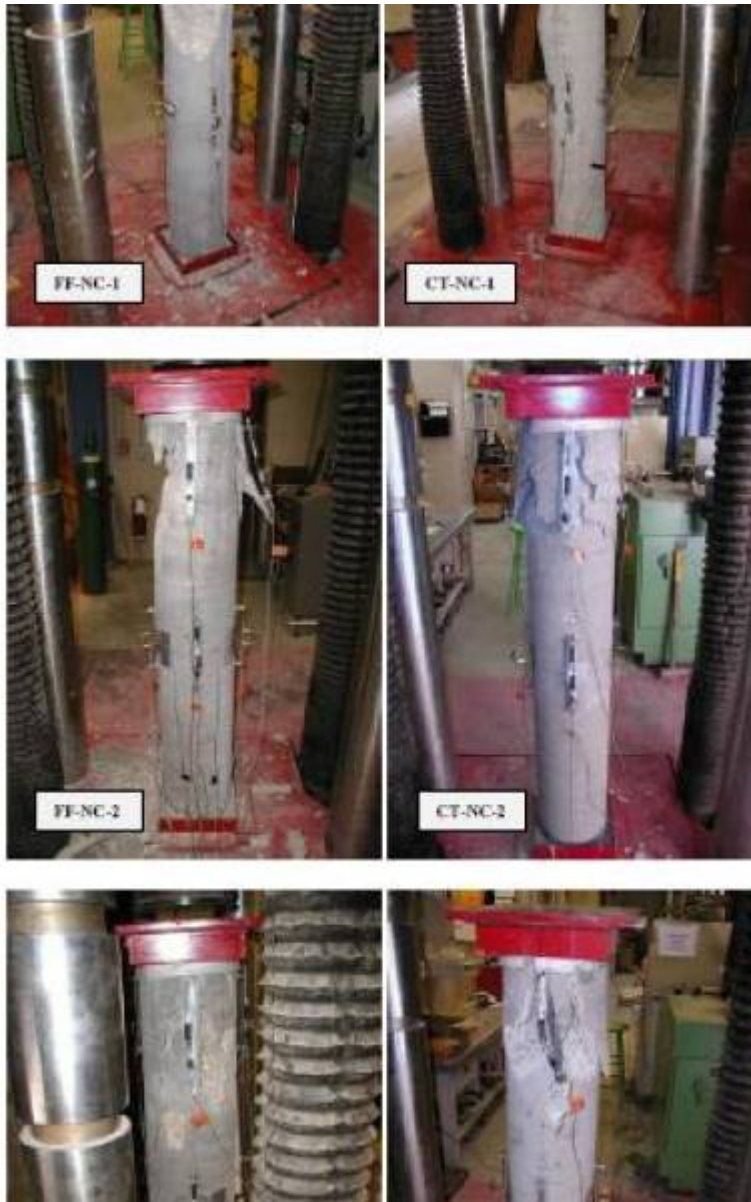
Figure 65: All columns after failure.
