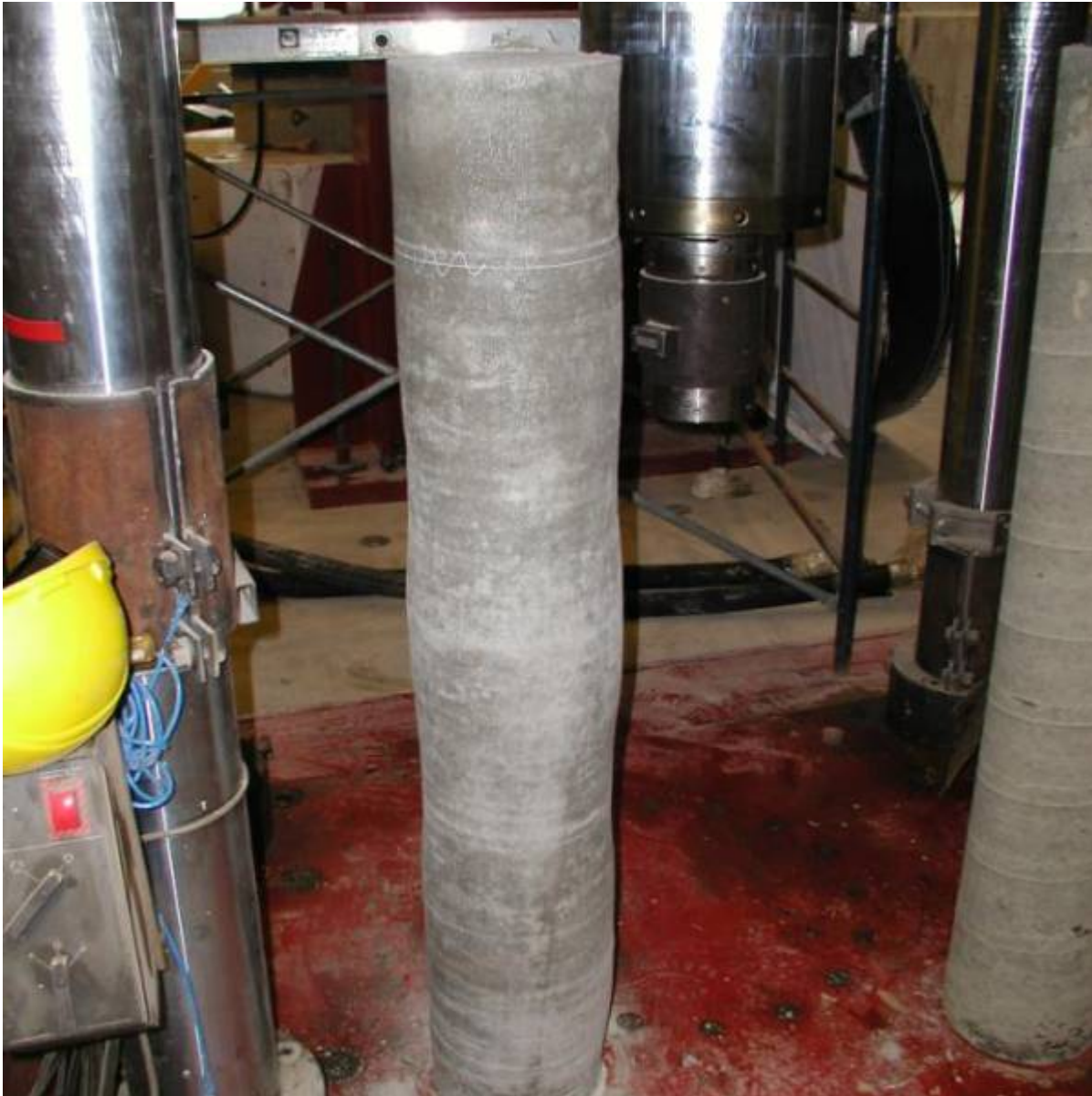
Figure 67: Bulged concrete column.
